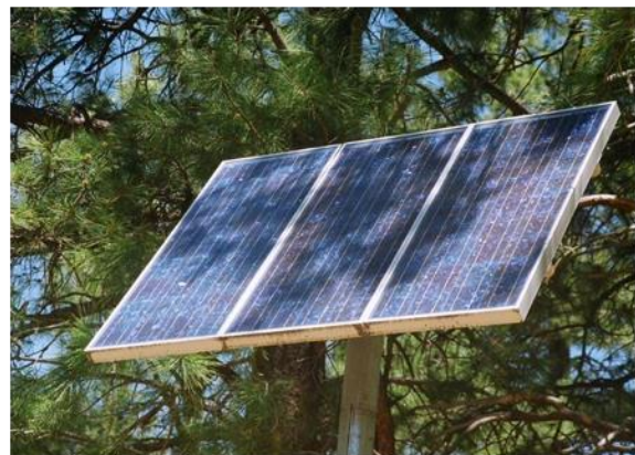
Fig. 1 Partial shading on the PV Panel
